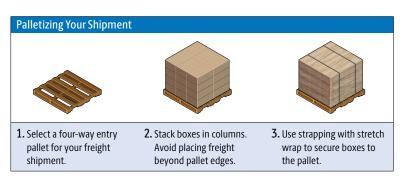
Pallets with four-way forklift entry are preferred as they help to improve handling and reduce damage to the shipment
